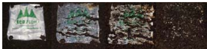
Time Lapse Approximately 4 Months
