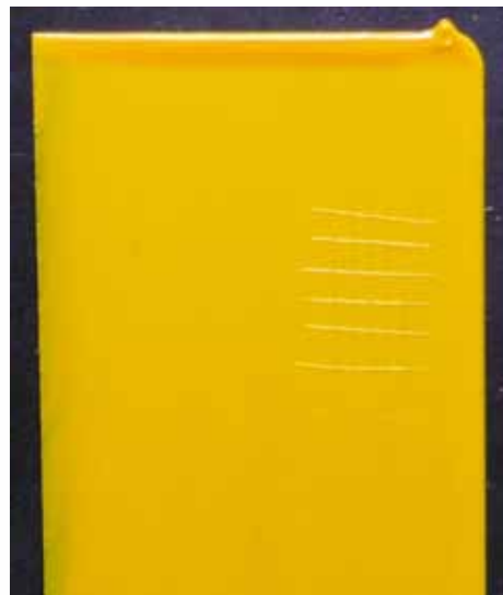
Panel cleaned with VpCI-429 and then coated with VpCI-386 Yellow
